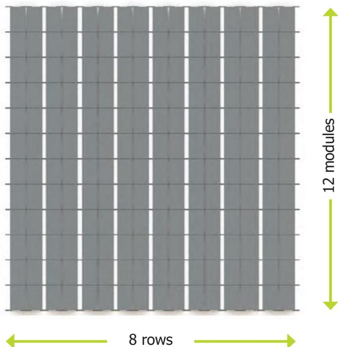
Maximum module array size: 8 rows with 12 double modules (192 modules).
