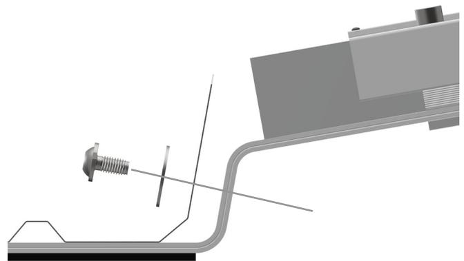
Place a building screen mat (PES, included in the scope of supply) on the left and right side underneath the ballast tray.
