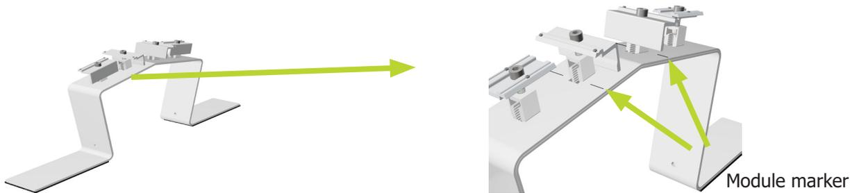
Example of the correct pre-assembly of the individual clamps on the bottom part.
