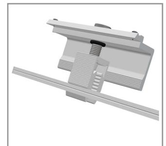
**Fastening to the mounting bracket with square cut-out**
