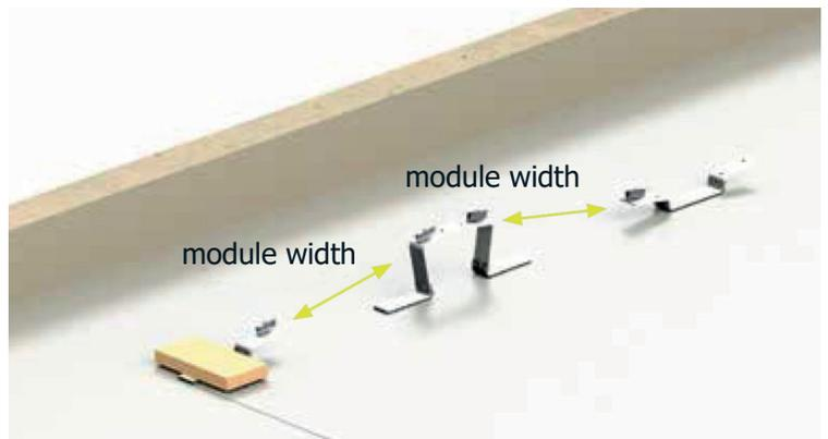
Place the front parts and connectors at approximately the required horizontal distance (module length). The exact distance is adjusted during installation of the module.
